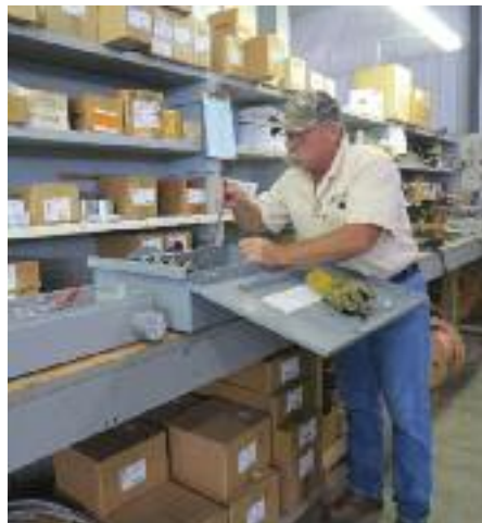
Garland Goracke, a warehouse clerk at Elkhorn Rural Public Power District, assembles a 3-phase meter loop.
