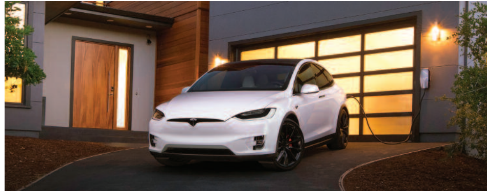
A Level 2 charging unit can provide about 250 miles of charge in 10 hours, making it a suitable charging solution. Photograph provided by Tesla
