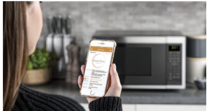
Smart microwaves like the GE model shown here include barcode scanning technology to allow product-specific cooking instructions to be sent to the appliance. Photograph provided by GE
